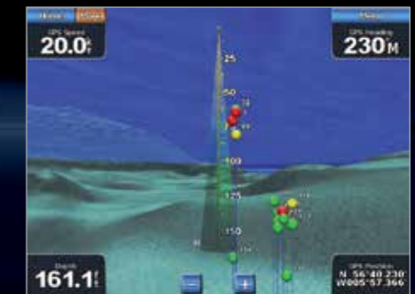
FishEye 3-D Underwater perspective view shows fishing target detected by connected GSD 22/24/26 sonar.
